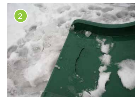
This tear could be an entanglement hazard.
